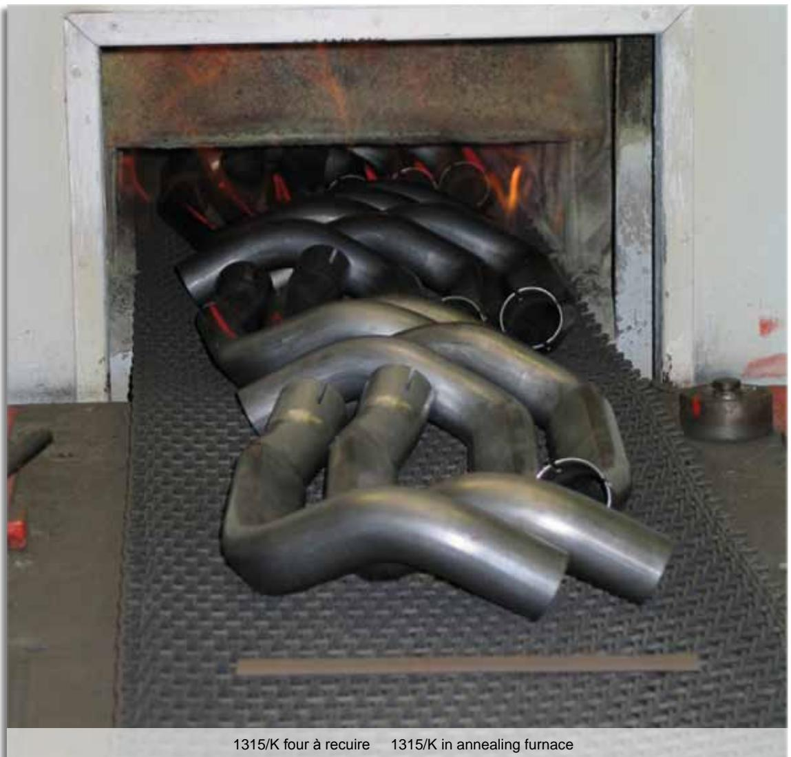
1315/K four à recuire 1315/K in annealing furnace
