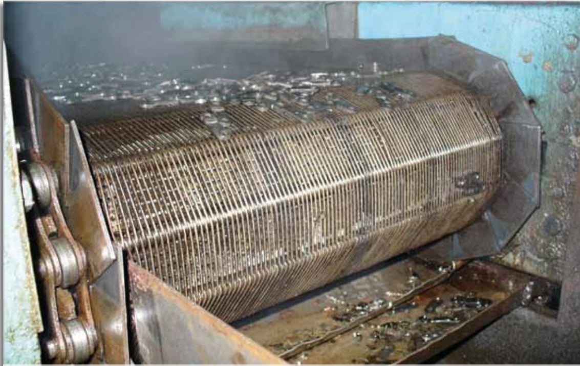
250,8/RZK inserts en U perforés 250,8/RZK with perforated U-inserts
