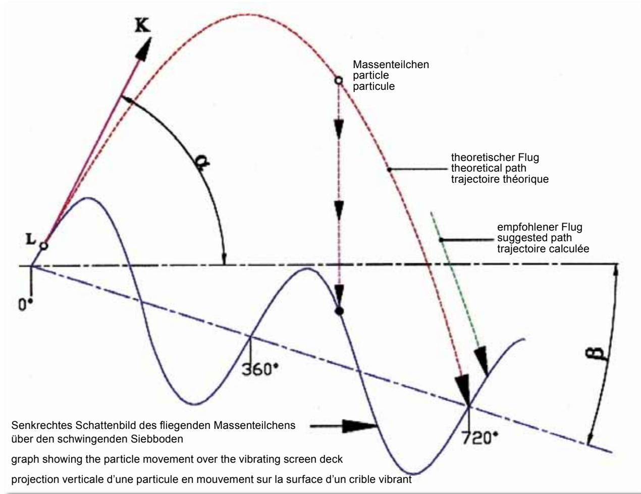
The dynamic parameters of the Delta 2 screening machine are designed that the throw of a particle is exactly two vibrations of the machine (circular motions).
