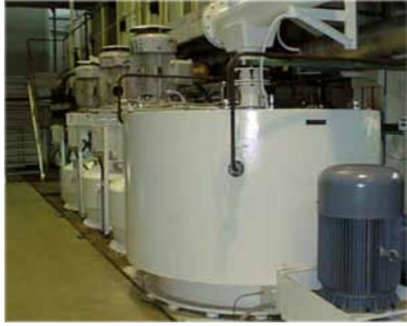
**HEIN, LEHMANN sugar centrifugals** are continuously operating centrifugals; available for discharging the sugar either dissolved or undissolved. A model with double stage basket allows pre- and afterpurging in one unit.
